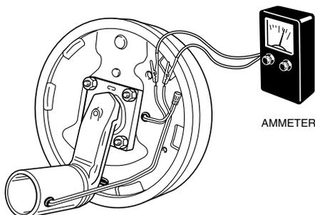
The most common electrical problem is low or no voltage and amperage at the brakes. Common causes of this condition are:
