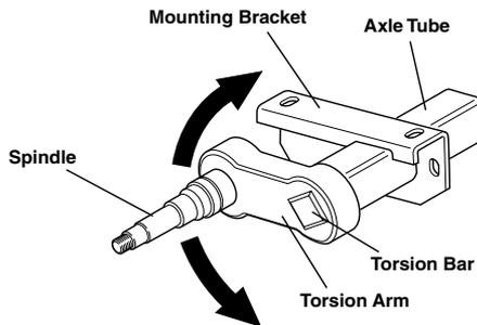
resistance in the rubber cords. This action provides the same functions as conventional sprung axles with several operating advantages including independent suspension.
